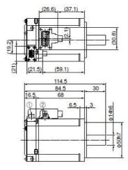
① Encoder connector ② Motor connector
